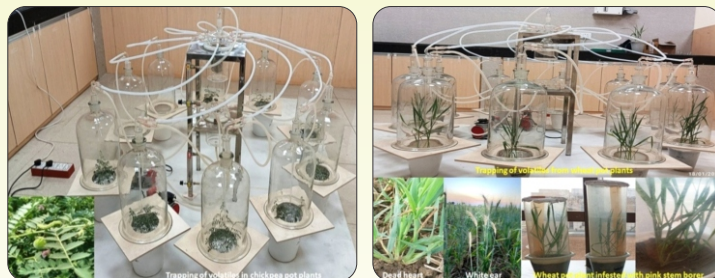
Fig 1.2. Trapping of volatiles induced by the borer pests of chickpea and wheat
